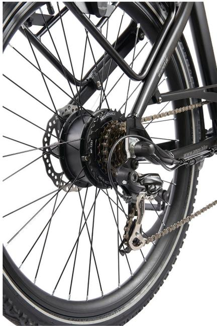
3.13.2 To change gear, use the 7 speed rapid fire gear shifter located on the right side of the handlebar. Push the lever to move up the gears 1 to 7, push the square button to move down the gears 7 to 1. Move one click at a time while pedaling to reduce stress on the gear change
