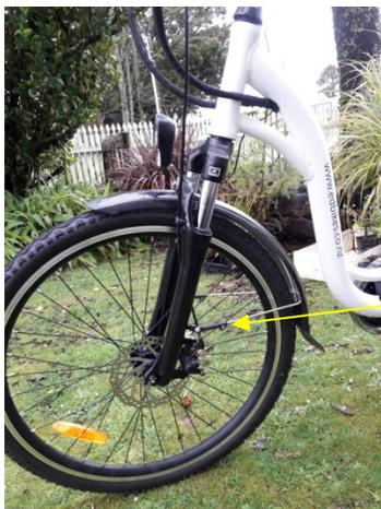
the eccentric lever it becomes very tight, the lever should face up the forks or towards the rear when it is in the lock position so as not to get caught on objects when riding
